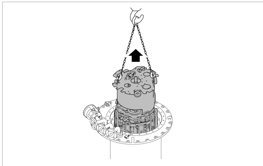
Figure 108: Lifting out diverter switch insert
